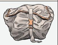
Completely latch bag to eliminate gaps
