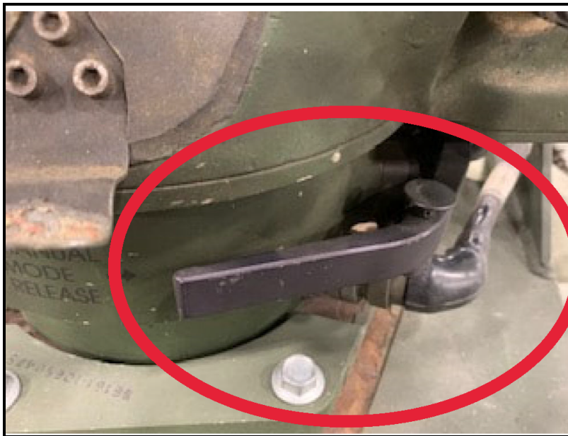
Azimuth clutch engaged
