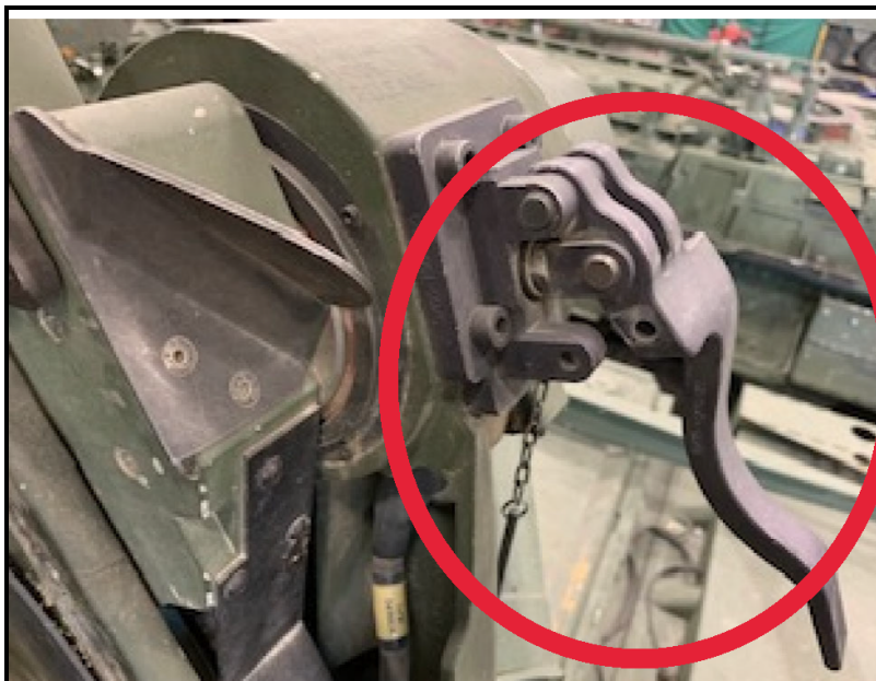
Elevation clutch disengaged
