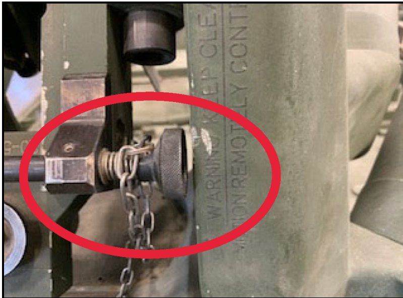
Properly installed rear weapon mount pin
