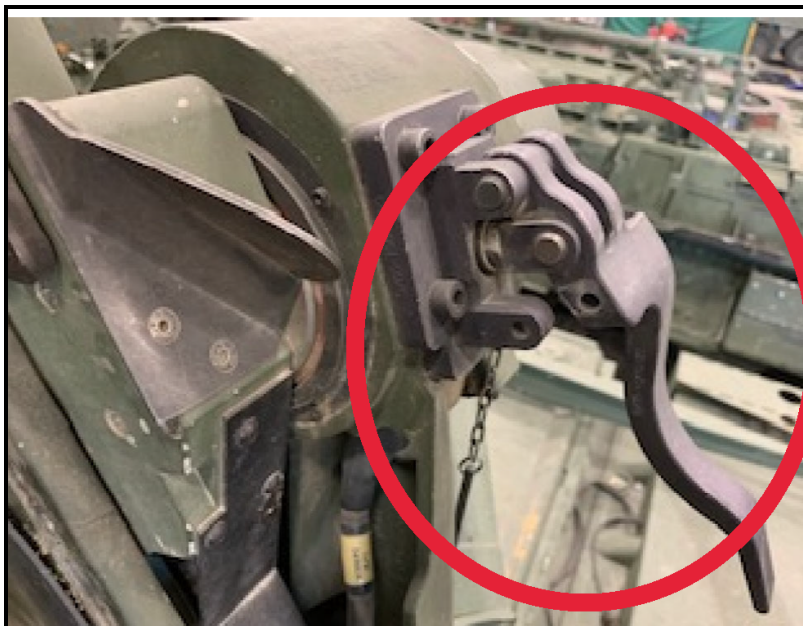
Azimuth clutch disengaged
