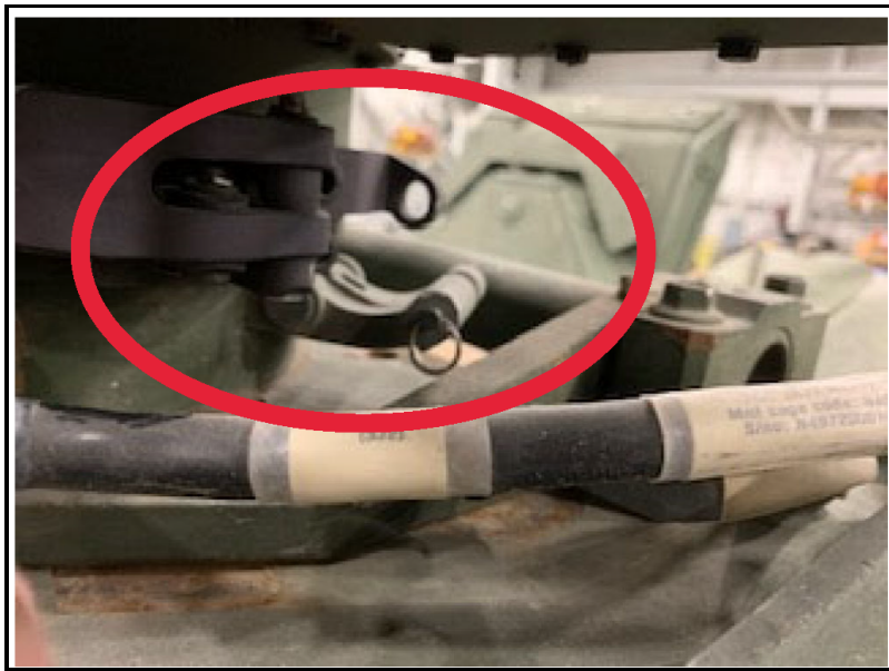
Be sure elevation lock is unlocked, in operation position before turning on RWS
