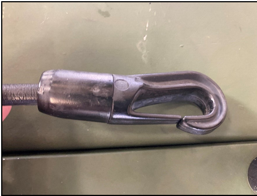
Inspect hook on end of cargo cover cord for damage
