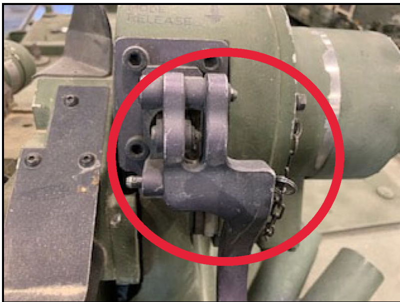
Elevation clutch engaged
