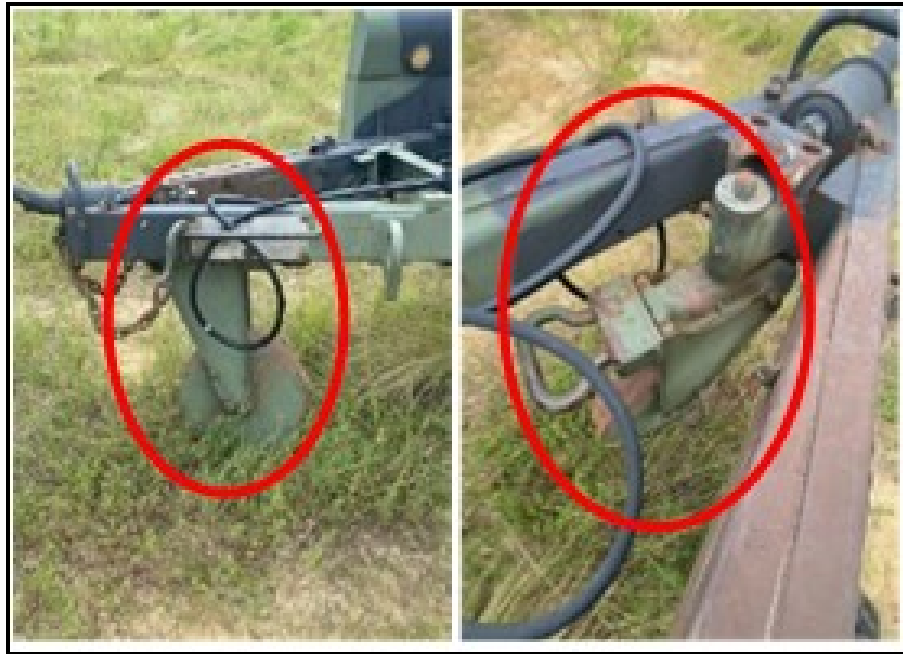
Non-adjustable caster is wrong landing leg
