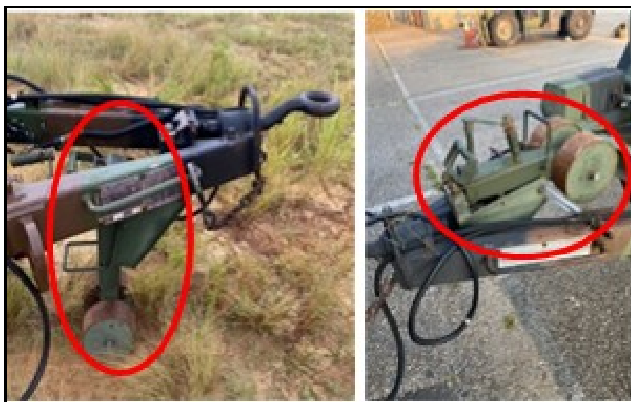
Use M149 adjustable caster landing leg
