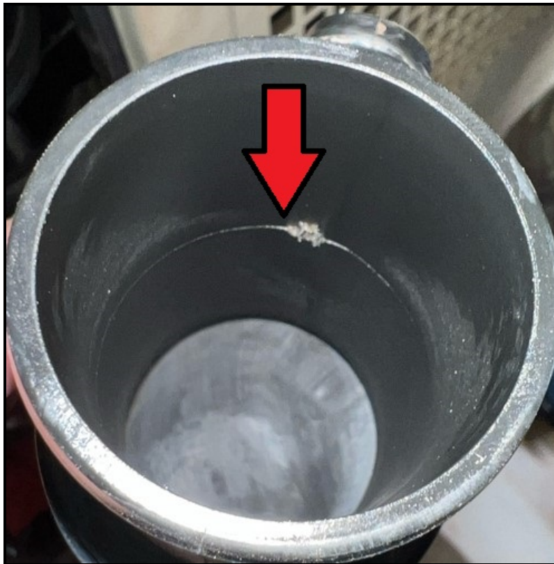
Oil breather joint blockage by fiberglass-like material
