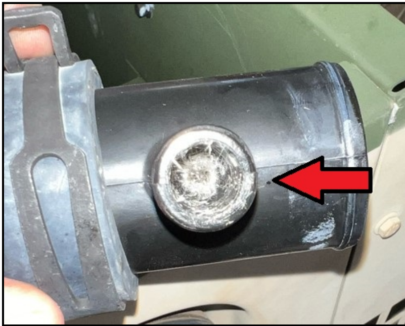
Check for clogged oil breather joint
