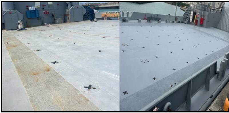
LCU2000 watercraft before corrosion removal (left) and after (right)
