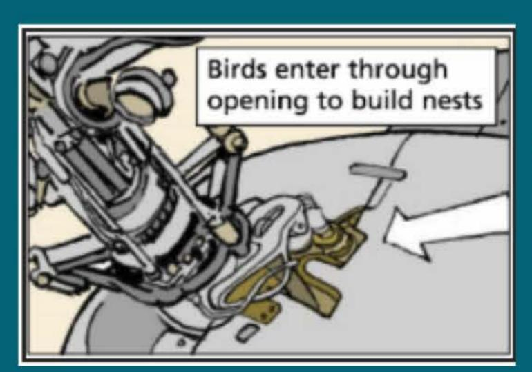
Birds like to squeeze through openings in the Apache's tail section. Inspect your aircraft for nest material because grass/twigs falling onto a hot gearbox could create a fire. While inspecting the tail rotor section for bird nests, remove the cover like it says in the TM 1-1520-LONGBOW/APACHE IETM (May 19). If birds have made your aircraft a home, see your canvas shop about making a cover for the tail rotor section. Learn more HERE.
