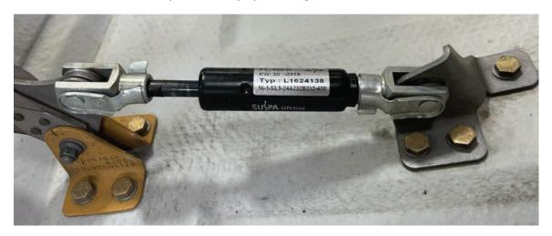
(f) Install the gas spring LH and the gas spring RH of the transmission cowling (2, Figure 803) as follows:
