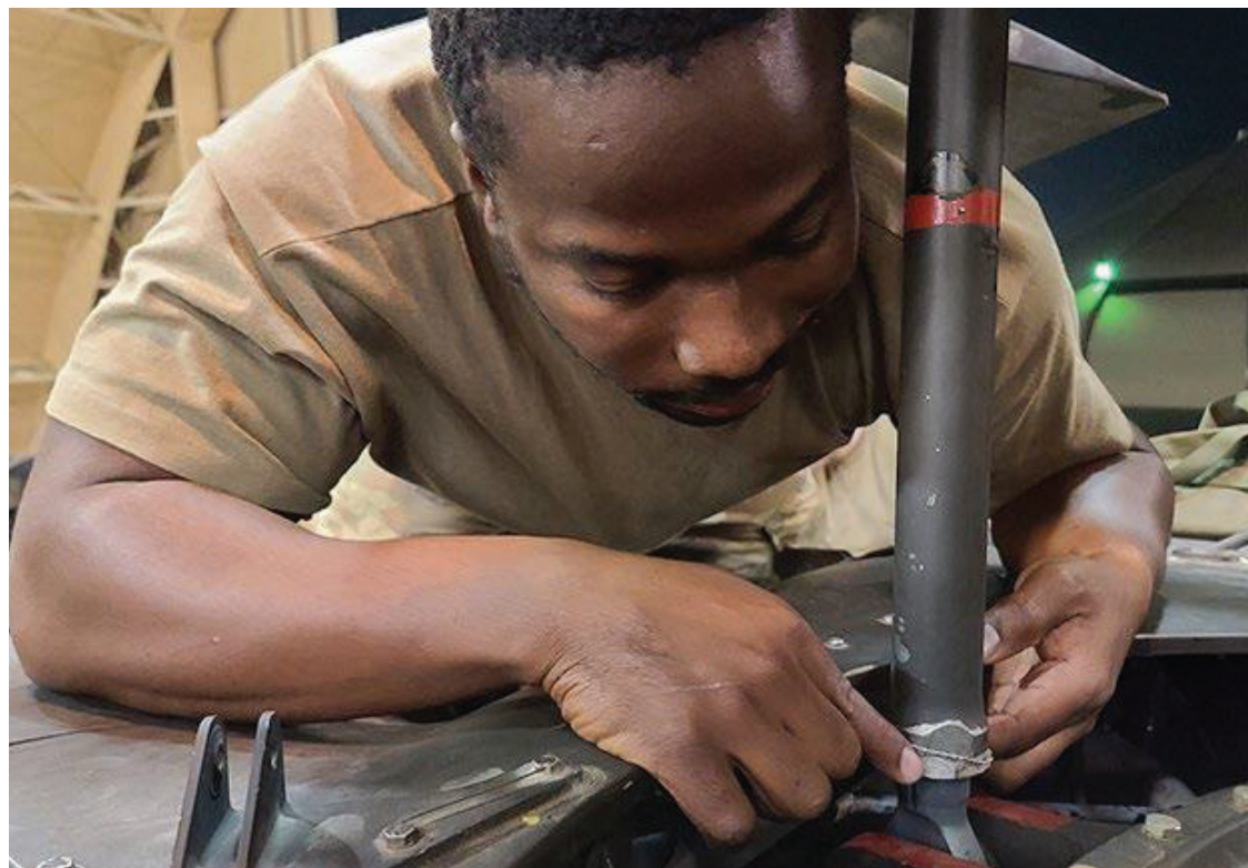
U.S. Army Staff Sgt. Leon Watson, a technical inspector with Bravo Company, 28th Aviation Support Battalion, 28th Expeditionary Combat Aviation Brigade, inspects a safety wire on a UH-60 Black Hawk helicopter at an airfield in the 28th ECAB's area of operations in the Middle East. (U.S. Army photo by Sgt. Francis Calabro)
