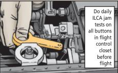
PURING OPERATION, THE RED JAM SENSOR INDICATOR BUTTONS WILL POP OUT AUTOMATICALLY IF THERE'S A PROBLEM WITH THE ILCA.
