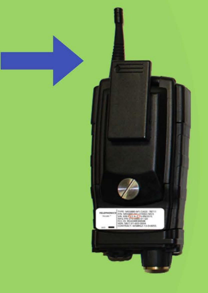
Inspect your aircraft now and record the software being used on the handheld enhanced mobile equipment (EME) and the integrated aircraft interface unit (IAIU) located on the main EAWIS hub in the cabin overhead. Submit that information to PM Air Warrior (PM-AW) to make sure the systems have the latest software.
